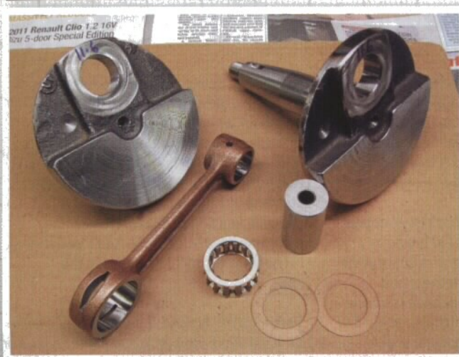
Most two-stroke cranks consist of a pair of webs, a crankpin, big end bearing and con rod. In this case the big end also has two shims which aren't used on all cranks.
