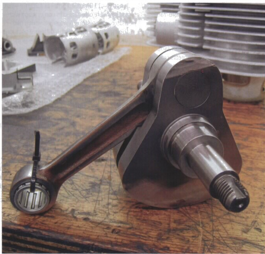
A custom crankshaft for reed valve engines produced by Scooter & Service in Hamburg.
