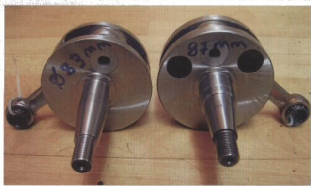
The long-stroke crank on the right has larger diameter webs and requires crankcase machining to suit.
