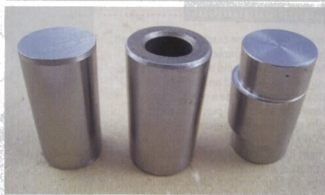
Crankpins (L-R): solid, hollow, eccentric.
