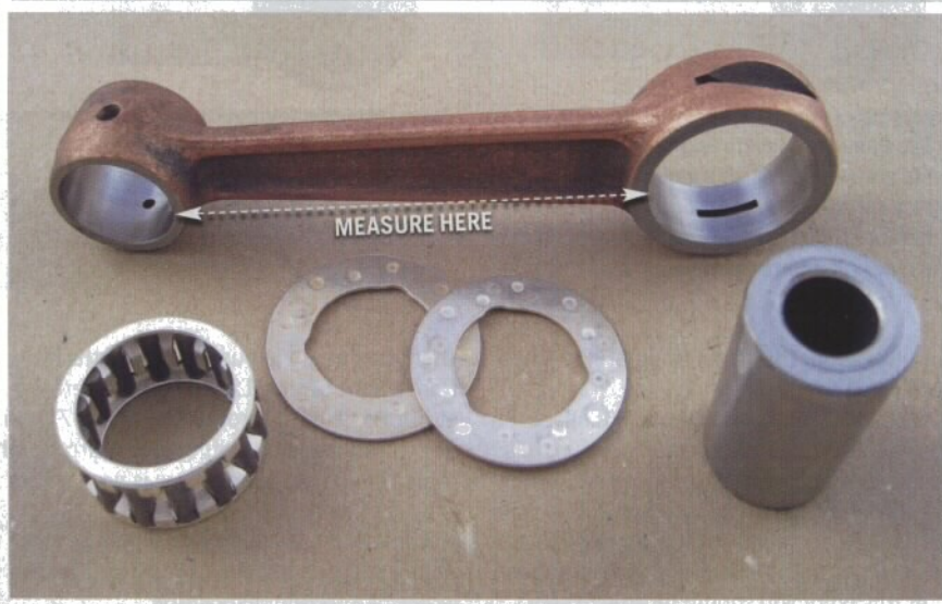
Con rods lengths are given centre-to-centre. Measure as shown and add half the diameter of each bearing hole to calculate the stated length.
